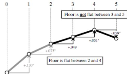
In a like manner, you can see that the portion of the floor spanned by Dipstick® readings #4 and #5 is *not at all flat*. The difference between Dipstick® readings #4 and #5 is
